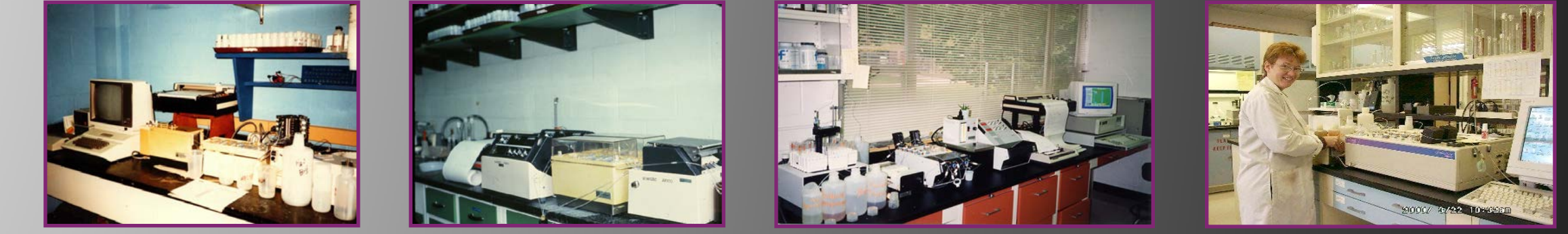
Automated Colorimetry Segmented Flow 1978-1985 Technicon Instruments Cl, NO 3 , SO 4 , PO 4 , & NH 4 Automated Colorimetry Segmented Flow 1978-1988 Technicon Instruments 2 systems added in 1982 Cl, NO 3 , SO 4 , PO 4 , & NH 4 Flow Injection Analysis 1989-1996 Lachat Quick Chem IV NH 4 & PO 4 Flow Injection Analysis 1996-2015 Lachat Quik Chem 8000 NH 4 & PO 4
