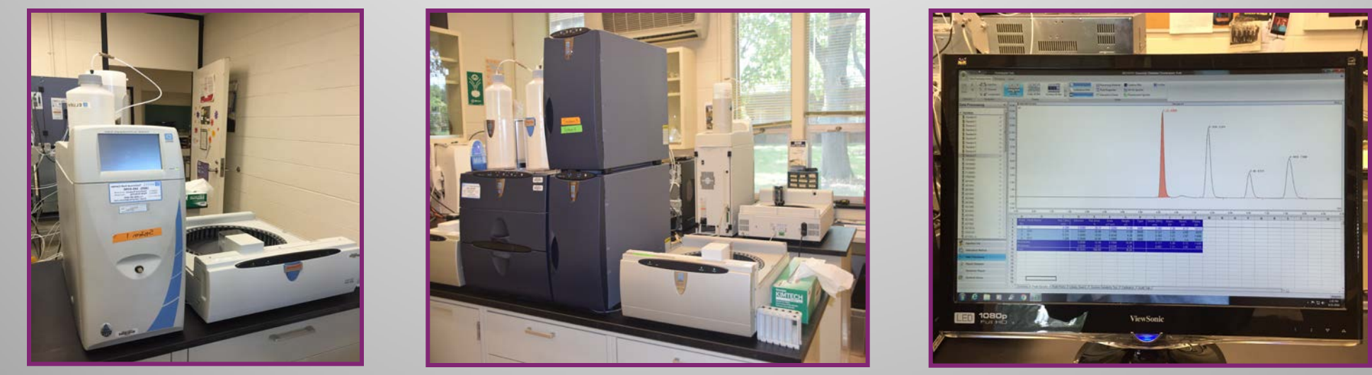
Ion Chromatography 2005-2016 Dionex Model ICS-2000 2 systems Cl, NO 3 , SO 4 , & Br Ion Chromatography 2011-2016 Dionex Model ICS 5000 2 systems Cl, NO 3 , SO 4 , & Br Dionex Chromeleon 7.0 Data Management Software 2011-2016
